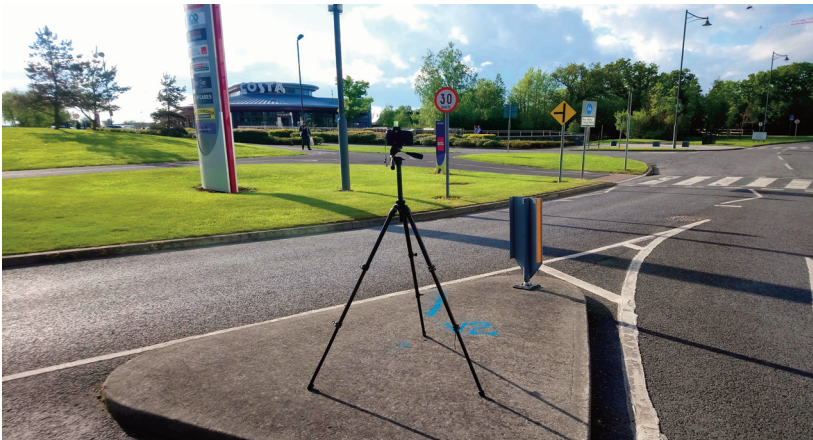
CAMERA SET UP Camera leveled and centred above surveyors mark
